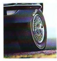
Tires. Included are Fiberglass Belted F70-14's with extra-narrow whitewalls; white sidewall 7.35 or E78-14's. Also available: widetread radial ply FR70-14's with narrow white sidewalls, Wheel Covers. Extra razzie-dazzie with full wheel covers in either 5-spoke design or wire style.
